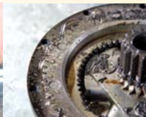
The gearbox had gaskets in all the critical mounting locations, but unfortunately it didn't hold out water during our test. As we split the gearbox, it let out a dribble of water and droplets were found around the gears as well
