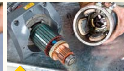
The motor showed signs of taking in water, but all that remained were a few droplets. The drain holes on the motor housing did their bit to let the majority of water back out
