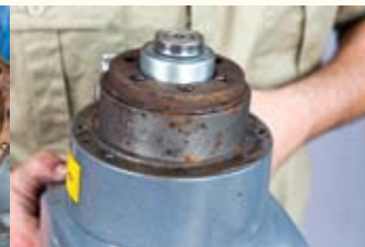
The gearbox was fitted with gaskets where the body meets the endplate and drum, which all seemed to be intact. They still managed to let in a slight amount of water. There were also traces of water around the external brake once the end cap was removed
