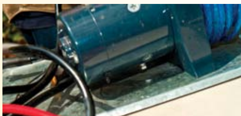
While it was clear the motor enjoyed its bath in the river, the drain holes did their bit releasing water the whole time during removal of the winch
