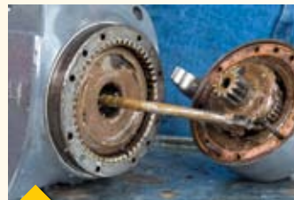
The gearbox was fitted with gaskets where the body meets the endplate and drum, which all seemed to be intact. They still managed to let in a slight amount of water. There were also traces of water around the external brake once the end cap was removed
