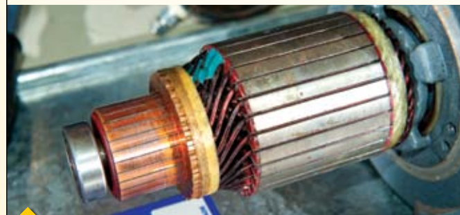
The drain holes worked a treat on the Premier's motor, as it was one of the driest coming out of the submersion tests. The only signs of water we could find were some slight traces of surface moisture on the inside of the motor body
