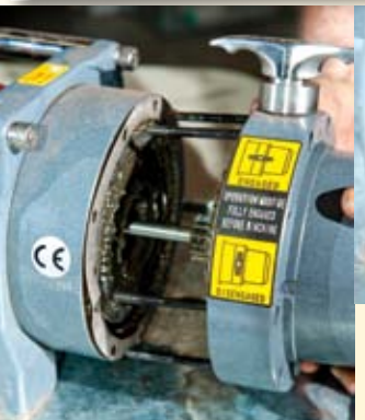
The gearbox sealed up well keeping water out of the grease and vital gear mechanism. A minor amount of water drained out through the bolt holes once the gearbox was split apart
